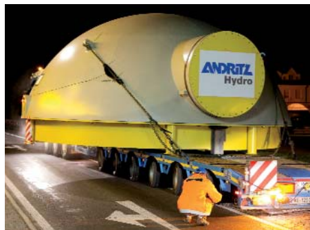
The power station components were around eight metres wide. That called for numerous traffic routing measures.
