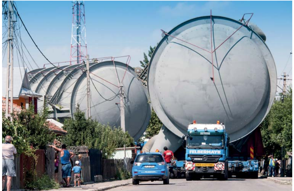
Due to the total height of 12.5 metres, countless overground cables that crossed the roads had to be switched off and temporarily dismantled – a complex undertaking. However, this meant that we were able to ignore the minimum clearance.
