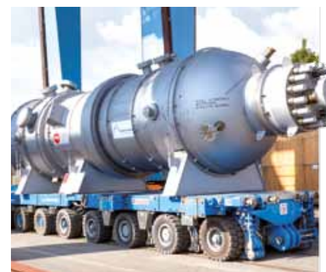
A 150-ton high-pressure heat exchanger was also shipped.
