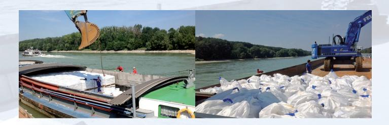
A motorised freighter that had run aground in Vienna's Freudenau power plant was lightened thanks to Horst Felix being deployed. To this end, around 400 tonnes of artificial manure had to be unloaded from the damaged ship to Horst Felix. Then, the motorised freighter was pulled into free water and the big packs were re-loaded with the cargo.
