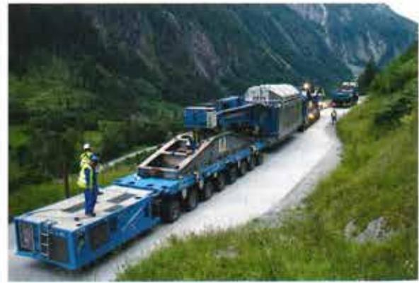
Fig. 2. The almost 40 m long total combination shortly before reaching the entrance of the tunnel. A strong performance in spite of the 12% gradient (Photo: Verbund/Schweinöster)
