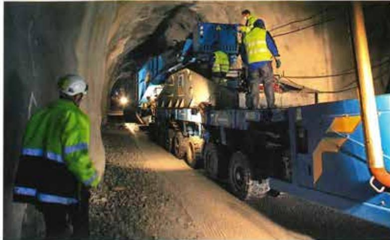
Fig. 3. The mobility of the SPMTs allows easy manoeuvring due to the steering angle of  $+130^{\circ}/-100^{\circ}$  (Photo: Verbund/Schweininöster)
