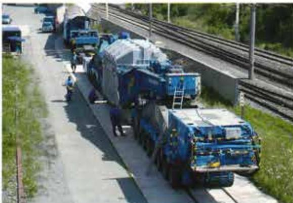
Fig. 1. Moving the 220 t transformer onto 16 axle lines of the Scheuerle SPMTs at the Maishofen railway terminus (Photo: Verbund/Schweinöster)
