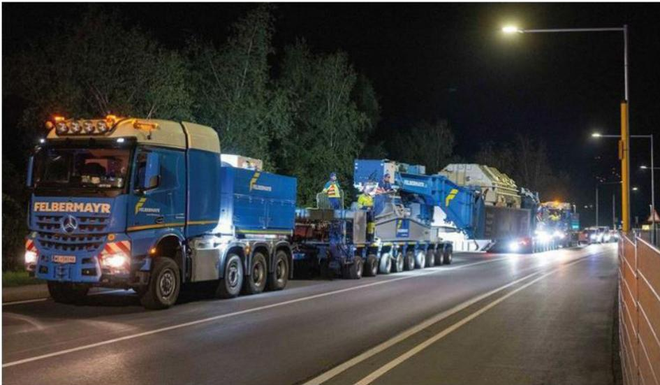
The transformers were then reloaded onto trailers for the final leg of the project. “In order to keep the traffic obstructions to a minimum, the stretches covered by road were carried out at night. The first stage began by driving through the Landec pedestrian zone. Including the tractor and pusher units, the heavy transport combination was 70 m long.
