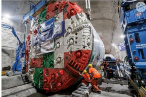
Once built, each of the tunnel boring machines weighed an “almost unimaginable” 2,000 tonnes complete with the trailer, Felbermayr said.
