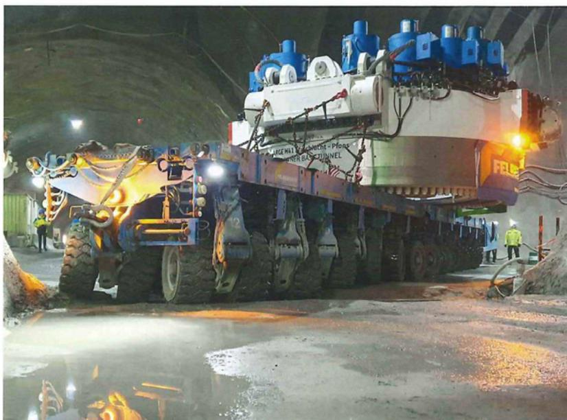
we reached the mathematical limit of the brakes, so in order still to safely carry out these transports we used a four-axle heavy-duty tractor as an additional braking vehicle," continues Meusbürger. "It took us roughly three hours to cover the first three kilometres with the steep gradient, and five hours to complete the entire route."
