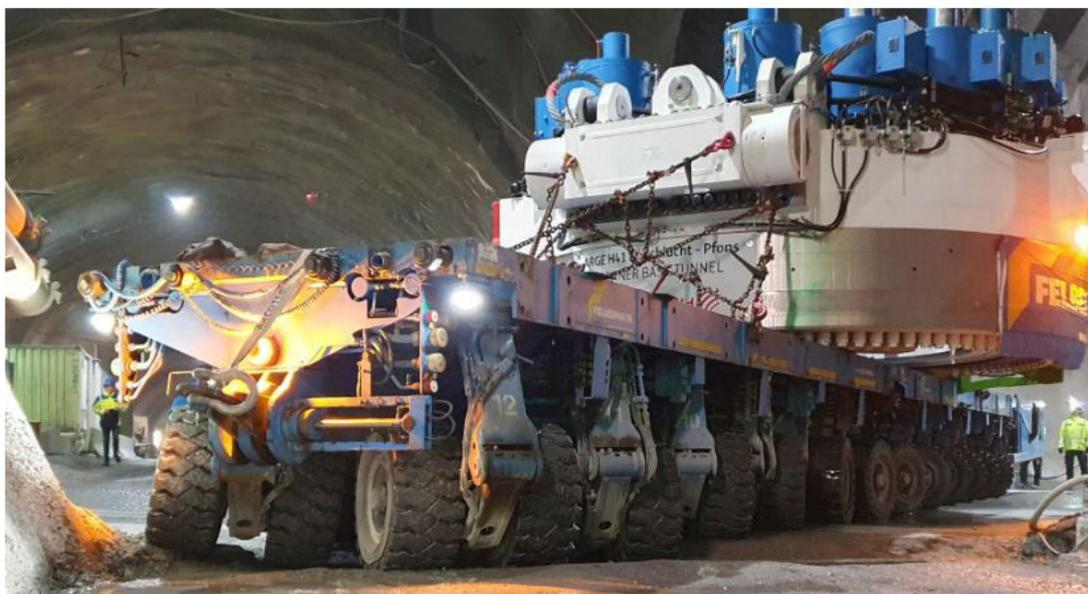
Heavy transport equipment specialist Felbermayr has transported two gargantuan tunnel boring machines for the construction of Europe's 55-kilometre-long Brenner Base Tunnel, the world's longest underground rail corridor.
