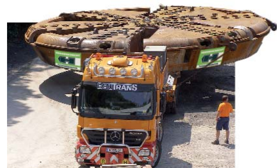
The heart of the tunnelling machine: a cutting wheel with a diameter of twelve metres, weighing 200 tonnes.
