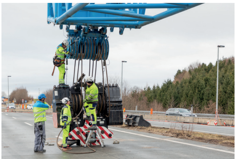
Each of the two hoist ropes of the LR 11000 has a length of 1,450 m and weighs around 7.4 tonnes
